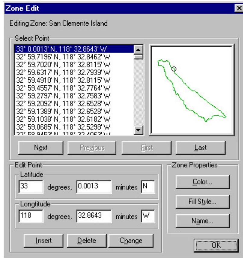
The Zone Edit Dialog Box is used to edit [zones](#). The large window at upper left shows the latitude and longitude of points on the perimeter of the zone. The highlighted point, which can be selected by clicking on it with the left mouse button, is the *current point* in the current zone. The large window at upper right shows the zone as it will appear on a [map window](#). The black circle in this window indicates the location of the current point.
