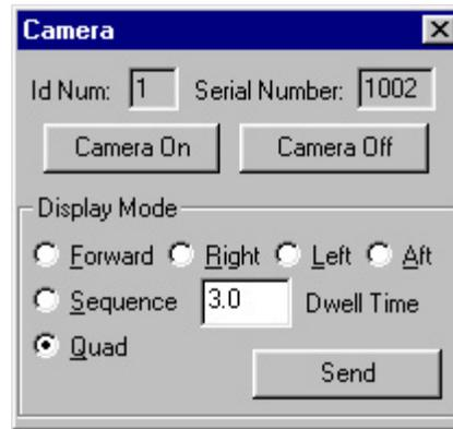
The Camera Dialog Box sends commands to the camera mounted on the [current target](#). The Identification Number and Side Number (Serial Number) of the current target are displayed at the top of the dialog box. The current target must contain a camera module for these commands to work.
