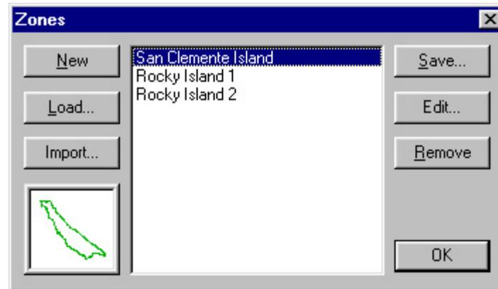
The Zones Edit Dialog Box is used to load, save, delete, create, and edit [zones](#). The large window at the center of the dialog box shows the currently loaded zones. The highlighted zone is the *current zone*. The current zone can be selected by clicking on it with the left mouse button. The small window at the lower left of the dialog box shows the current zone as it will appear on a [map window](#).
