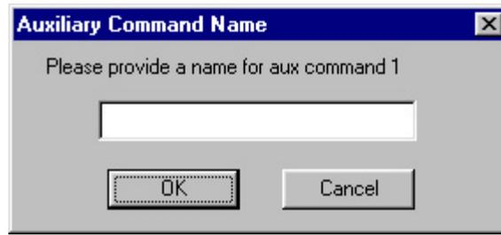
The Auxiliary Command Name Dialog Box records a name for one of the auxiliary commands. Enter the desired name into the edit box, then click on OK. This name will then appear on the [Auxiliary Command Dialog Box](#).
