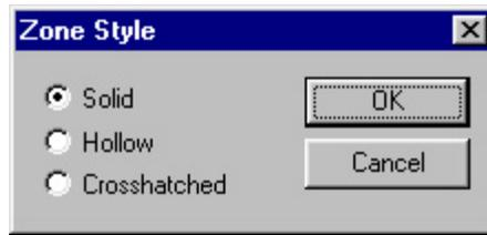
The Zone Style Dialog Box is used to set the [zone](#) drawing style. A zone may be solid, hollow, or crosshatched. For example, the following [map](#) shows a solid blue zone, a portion of a hollow green zone, and a crosshatched red zone.
