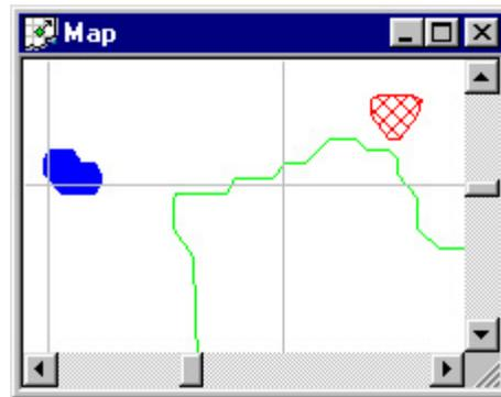
Zones can be created, edited, saved to a file, and loaded from a file using the [Zones Dialog Box](#), which can be displayed by selecting Zones from either the [Settings Menu](#) in the [Pre-Mission Menu Bar](#) or the [Settings Menu](#) in the [Mission Menu Bar](#). Each zone may be drawn in a different color, and may be either solid, hollow, or crosshatched.
