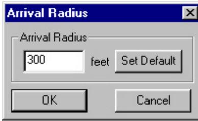
The Arrival Radius Dialog Box sets the *arrival radius*, which is the distance from the center of a waypoint in a [maneuver](#) at which a target is deemed to have arrived at the waypoint. Enter the desired arrival radius in feet in the edit box and click OK. Click on the Set Default button to set the default recommended arrival radius. Making the arrival radius smaller will not make the navigation more accurate, as the target vehicle will always aim for the center of the waypoint.
