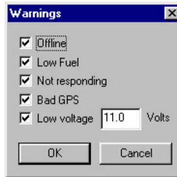
The Warnings Dialog Box allows the operator to choose which conditions the operator will be warned about. There are five warning conditions:
