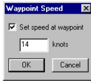
The waypoint Speed Dialog Box sets the speed that the [current target](#) is to take on at the [current waypoint](#). The ROS will then automatically issue a Speed Command to this the when it arrives at the waypoint. The checkbox is checked if this function is required, and unchecked if it is not required. The edit box contains the desired speed in knots.
