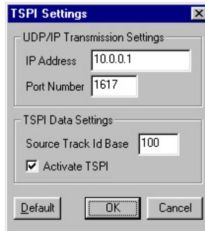
(NetROS only) The TSPI Settings Dialog Box manages the TSPI settings. Two edit boxes at the top of the dialog box contain the IP address and port number of the computer receiving the TSPI packets. The third edit box contains the *source track id base*, which is added to the identification number of each vehicle in the TSPI packets. The checkbox is checked if TSPI packets are to be sent (in which case TSPI packets are sent during both simulations and live missions), and unchecked otherwise.
