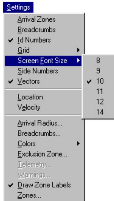
(NetROS only.) The Settings/Font Size Menu is accessible from the [Settings Menu](#). It has six selections, each of which set the screen font size for the [current window](#) (this includes data written beside the vehicle [icons](#), [zone](#) labels, and grid labels):
