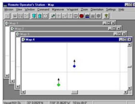
At the top of the ROS window is a [Mission Menu Bar](#) consisting of ten pull-down menus which are used to control the
