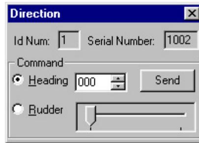
The Direction Dialog Box sends Heading and Rudder Commands to the [current target](#). The Identification Number and Side Number (Serial Number) of the current target are displayed at the top of the dialog box.
