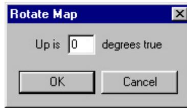
The Rotate Map Dialog Box is used to rotate the [maps](#) in the ROS window. This operation applies to all maps.
