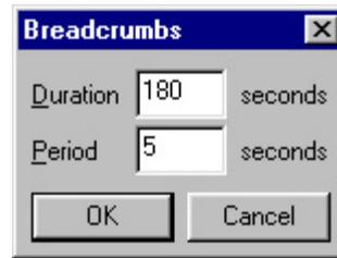
The Breadcrumbs Dialog Box sets the duration of the breadcrumbs (the amount of time that each breadcrumb exists) and the period of the breadcrumbs (the amount of time between the creation of each breadcrumb by an individual vehicle).
