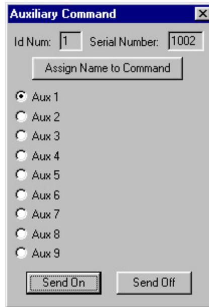
(NetROS only.) The Auxiliary Command Dialog Box sends an Auxiliary Command to the [current target](#). The Identification Number and Side Number (Serial Number) of the current target are displayed at the top of the dialog box. There are nine possible auxiliary commands that can be sent to the target. The action taken by the target in response to an auxiliary command will depend on what hardware is on board. Each Auxiliary Command has an On mode and an Off mode.
